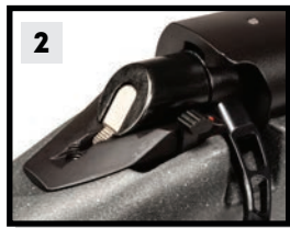
Cocking indicator on "fired" position
